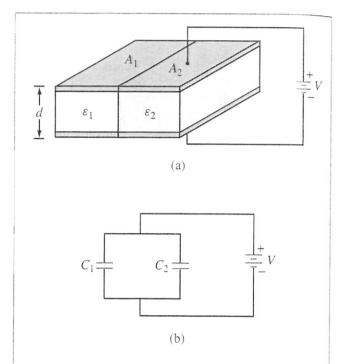
Figure 4-34: (a) Capacitor with parallel dielectric section, and (b) equivalent circuit.
