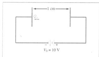
Figure 4-33: Electron between charged plates of Problem 4.50.
