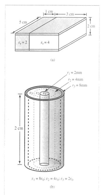
Figure 4-35: Dielectric sections for Problems 4.53 and 4.55.
