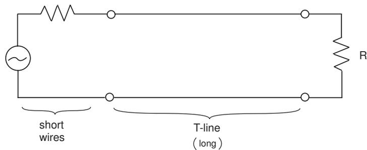
Figure 1.1: Circuit diagram symbol for a transmission line.
