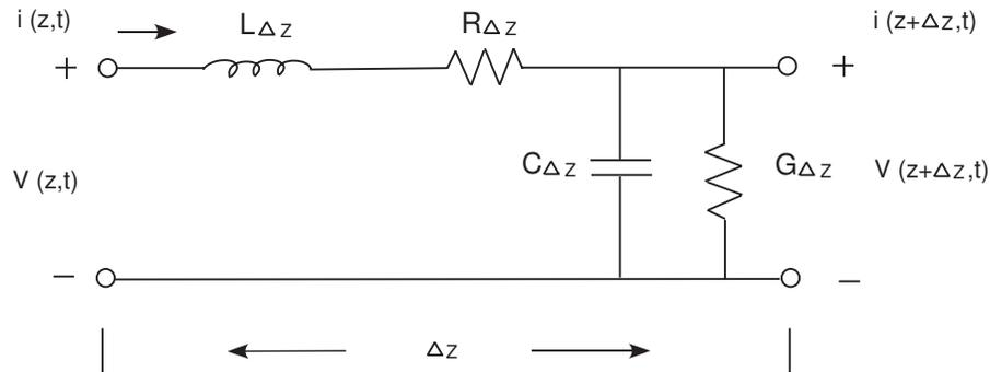
Figure 1.2: Lumped element model for a short section of a transmission line.
